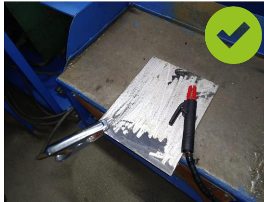
Figure-2 Grounding should be done close to the welding area
